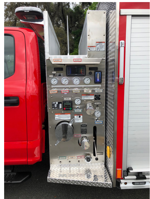
Two pre-connected crosslays and conventional mid-ship pump panel and controls.
