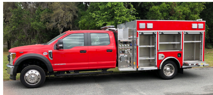
Large compartmentation provides storage for firefighting equipment; E-Tools and other rescue equipment; EMS medical kits, defibrillator and oxygen.
