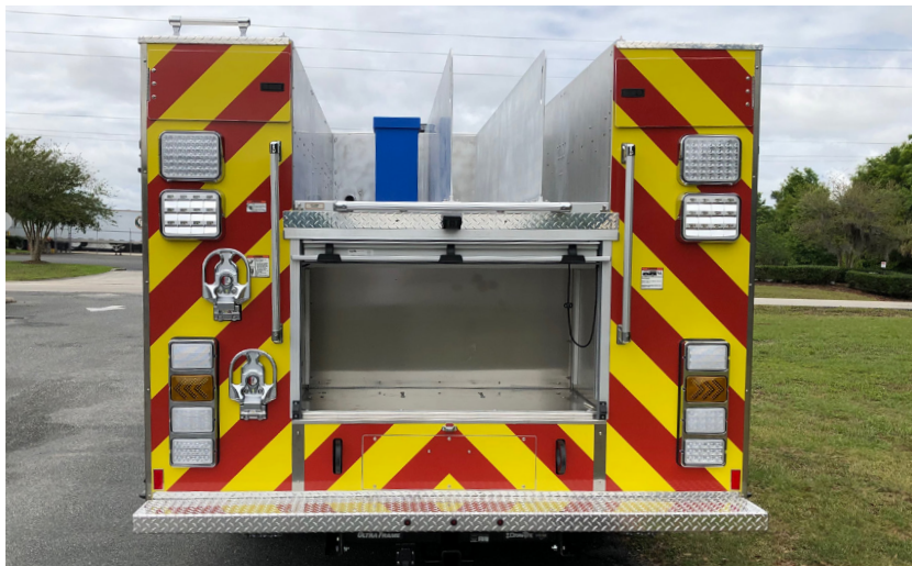
Rear compartment large enough to accommodate a booster hose reel. Upper, left and right ladder and hard suction compartments.
